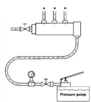
After completion of the pressure test all fittings are to be checked for possible leakage. The results of the pressure test must be recorded in a report as a record for the plumber and customer. The forms at the end of this chapter can be used for this report.
