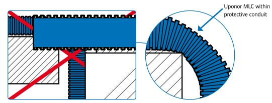
Pipes installed through ceiling recesses and wall cut-outs may never be bent over edges.
