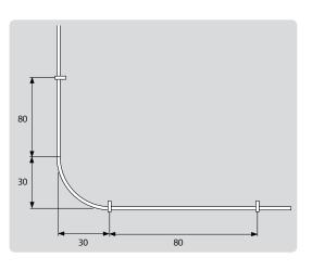
When installing Uponor MLC pipes on concrete floors a fixing distance of 80 cm is recommended. The pipe is to be fixed within a distance of 30 cm in front and behind each bend. Pipe crossings are to be fixed. The fixing can be done using a synthetic plugged hook for single or double pipe fixing.
